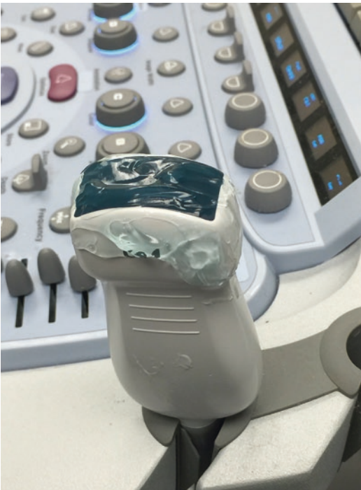
Fig. 3.1 Cleaning of all visible soil and contaminant should be done before any disinfection
