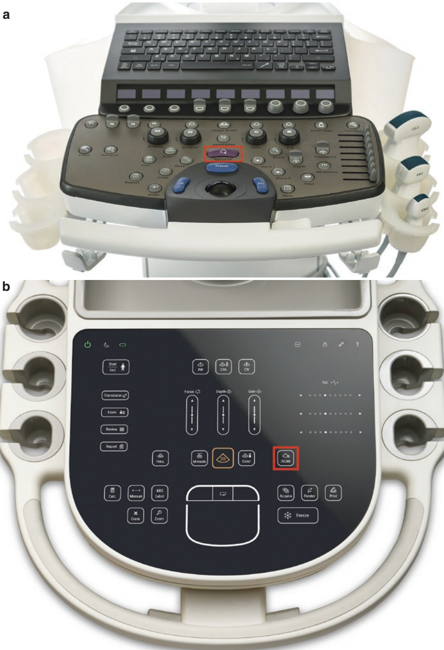
Fig. 2.15 (a, b) Optimization button automatically adjusts multiple settings to improve the image quality. Manufacturers can give the button a different name, but it
