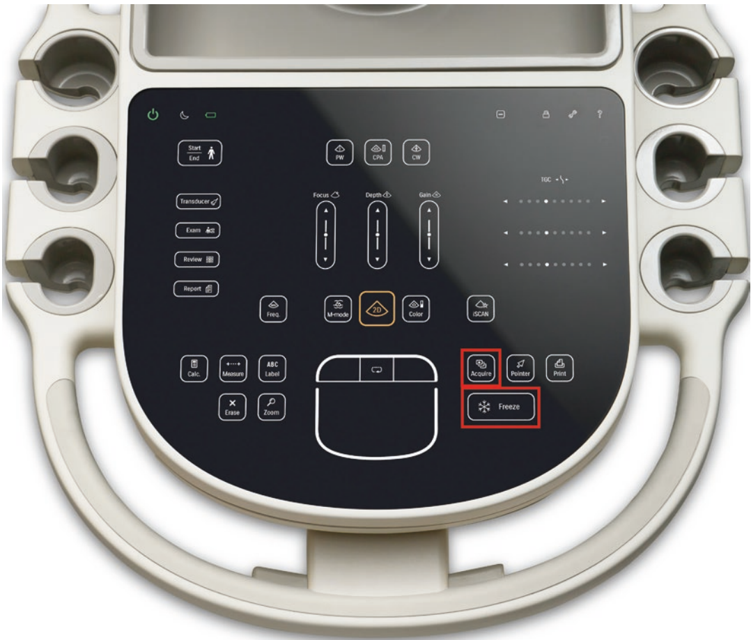
Fig. 2.16 The “Freeze” and “Acquire” (image saving) buttons on Philips machine
