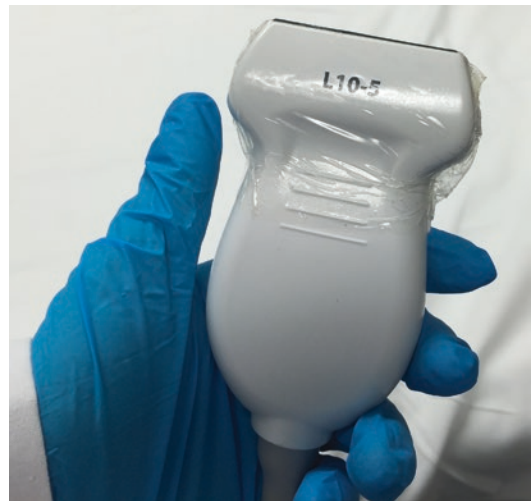
Fig. 3.9 The presence of air bubbles can reduce image quality
