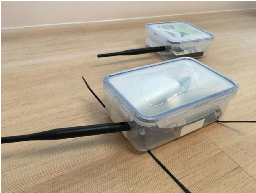
Fig. 1 Open-source environmental sensor mote
