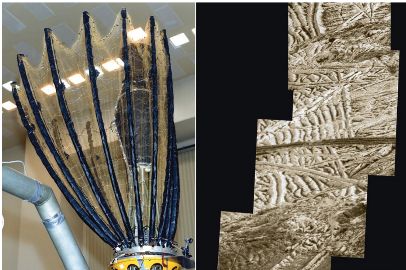
Fig. 3.10 Despite a fouled high gain antenna (JPL's flight hardware simulation at left), the Galileo mission returned spectacular images of the ice moons of Jupiter (Europa seen at about 12m/pixel, at right). (Images courtesy of NASA/JPL)
