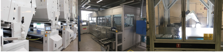
Fig. 2. Machine operators/technicians at company A, B and C need remote assistance to solve problems with different machines, including large printing machines at company A (left), special washing machine for molds at company B (middle), and bolt-lubing industrial robot at company C (right).
