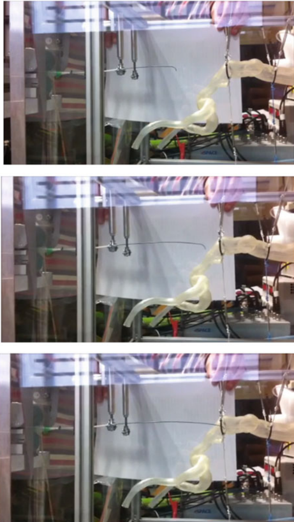
Fig. 8 Various stages of movement of the catheter based on remotely detected hand gestures
