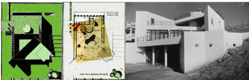
Fig. 4 Alberto T. Estévez, House M. , Almerimar, 1993–95. Green roofs, main floor with greenhouse turned 45° to face south, with water in the south, closed to north, with open side galleries, and lower floor half-buried and aerated
