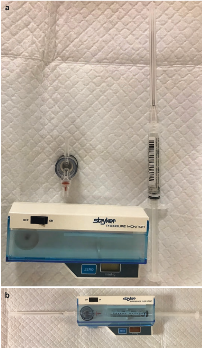
FIGURE 21.3 (a, b) Stryker device. Needle, monitor, syringe, and diaphragm. Needle, monitor, and syringe separate (a) and assembled (b)
