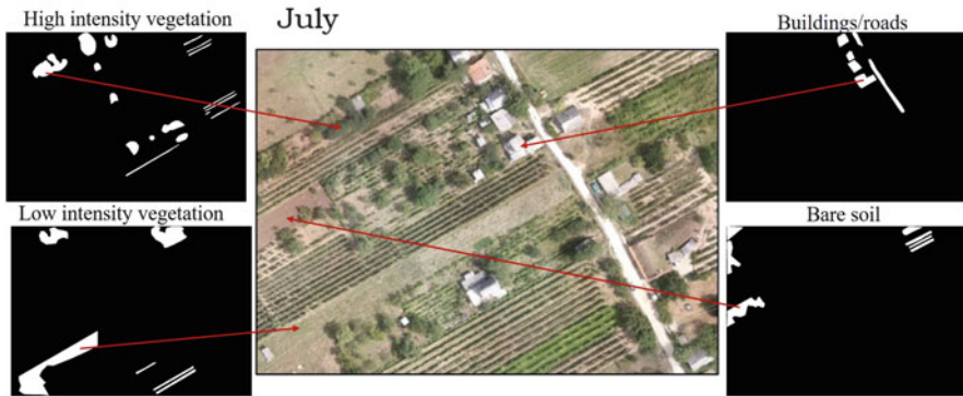
Fig. 4 Training masks used for supervised segmentation
