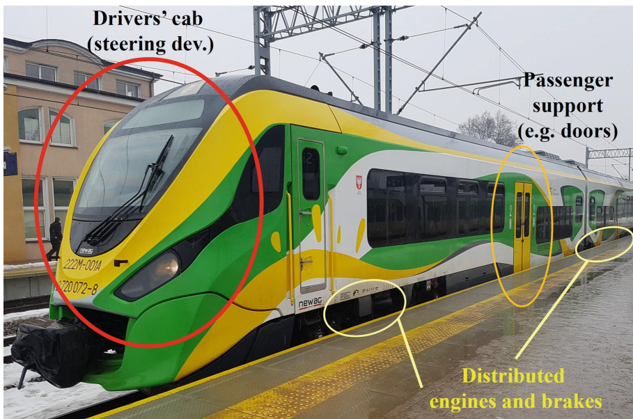
Fig. 2. Steering, driving & braking and passengers' support components Koleje Mazowieckie train at Siedlce station [own elaboration]
