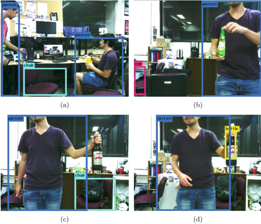
Fig. 3. Detection examples of tiny-YOLO ROS for Pepper-Jetson TK1, at \sim 4.8 FPS and input image size of 320 \times 320 . This resolution allows detection of people and medium to large size objects, while struggles with small ones (a) Correct detection of multiple objects. (b) Example of an incorrect car detection, false positives are infrequent. (c) Correct detection of a person and a chair, but the bottle is ignored. (d) Correct detection of a small object when moving bottle from (c) closer to the camera.
