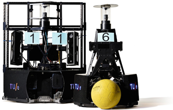
Fig. 1. Fifth generation TURTLE robots, with on the left-handside the goalkeeper robot. (Photo: Bart van Overbeeke)
