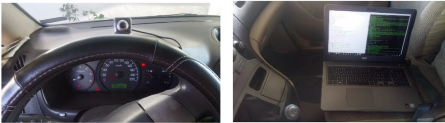
Fig. 5. Left: Mounting camera to our car dash for drowsiness detection. Right: Using a PC to run the actual drowsiness detection algorithm.
