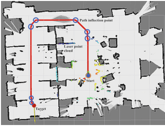
Fig. 9. Original A* algorithm results (Color figure online)
