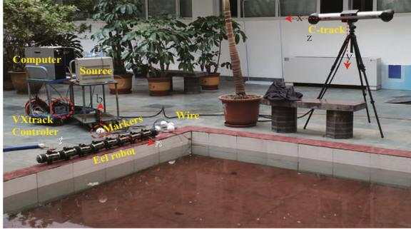
Fig. 4. Experimental equipments.
