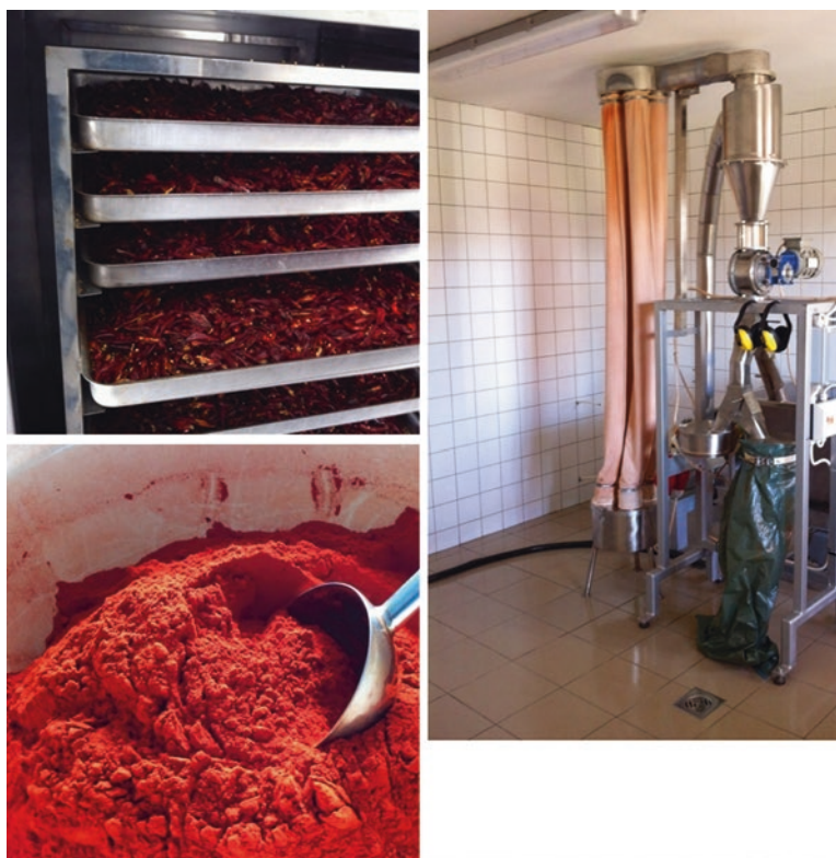
Fig. 8 Small scale paprika dryer, grinder and end product. (Source: SZABO, Peter, producer (5 ha area, 6 tons of ground paprika from Bátya, near Kalocsa))
