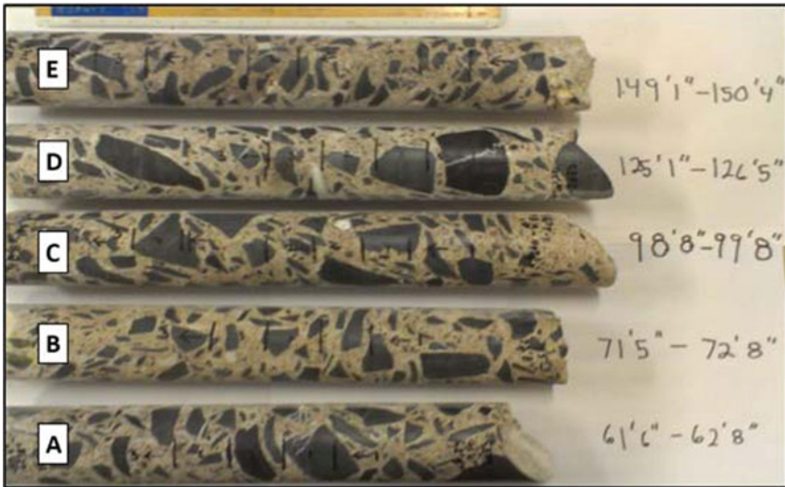
Fig. 6 Five concrete core samples (2.5" or 63.5 mm diameter) collected between depths of 20 and 45 m in borehole SEPI-1. Aggregate pieces are greywacke. Fractional porosities determined by hydrostatic weighing of three 30 mm thick disks from each sample varied from 0.11 to 0.16 ( \pm 0.02 )
