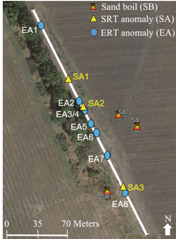
Fig. 12 An aerial image of survey line 3 (landside) with locations of SRT and ERT anomalies indicated along the survey line
