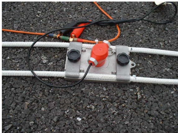
Fig. 4 A geophone on an aluminum plate of land streamer used in a surface wave method. The land streamer comprises 24–48 geophones on aluminum plates, respectively, aligned in series at 1–2 m intervals by two parallel ropes on the ground surface
