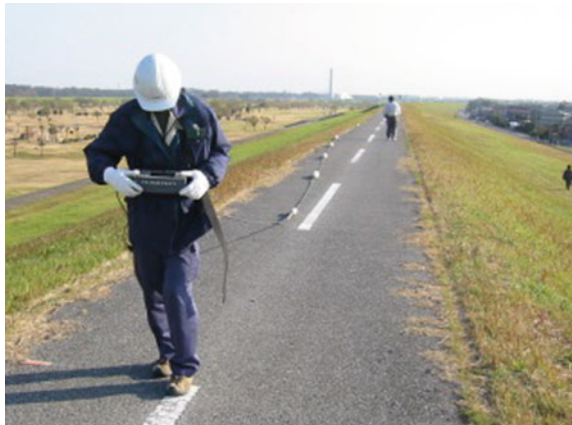
Fig. 5 Data acquisition of capacitively-coupled resistivity (CCR) method using Geometrics' OhmMapper
