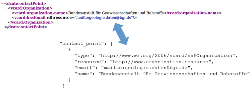
Fig. 4. Mapping of DCAT-AP to CDS and vice versa
