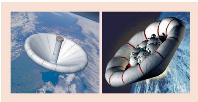
Fig. 30.3 Inflatable decelerator concepts. (Courtesy of the Inflatable Re-entry Vehicle Experiment (IRVE) Project)
