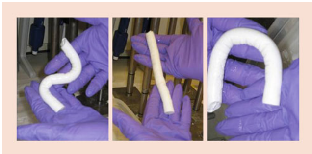
Fig. 30.6 A diisocyanate-reinforced wet gel with 35 mol% BTMSH-derived Si and 30 mol% Si from APTES is shown to be flexible and resilient before drying
