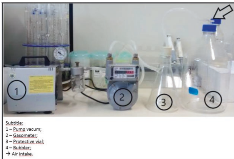
Fig. 8.3 Equipment for the sampling of air in liquid media. (Source: The Author)
