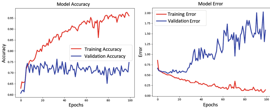
Fig. 3. Accuracy and error by epoch curves for the best model found for the classification of bacterial or viral pneumonia.
