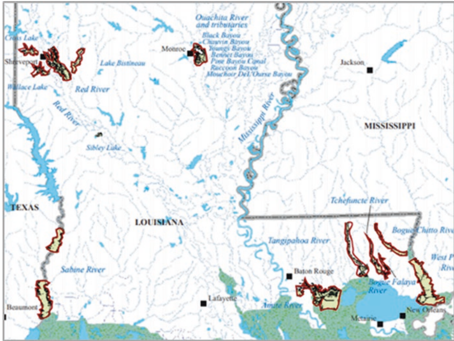
Fig. 1.6 To supplement DFO flood footprint for the March 2016 event, the flood polygons (yellow) in Watson et al. (2018) were traced (red) and combined
