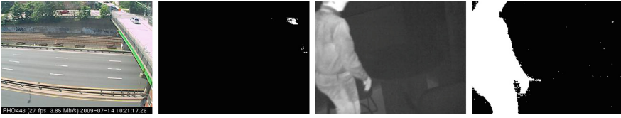
Fig. 3. A sample frame from Street Light (left) and Library (right) video sequences and the detected foreground object respectively.
