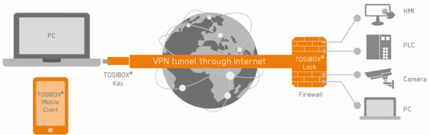
Fig. 3. An illustration of the main functionalities of Tosibox [32].
