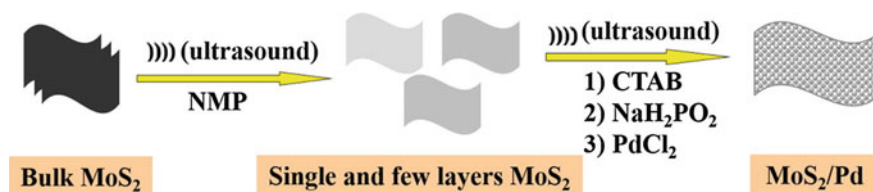
Fig. 9 Schematic design of the progress of fabrication process of sonochemical doping of Pd on MoS 2 to form MoS 2 /Pd composite [157]
