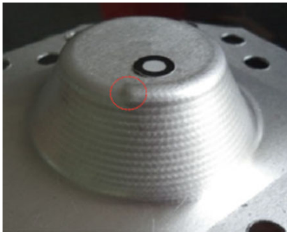
Fig. 8 Final manufactured part by SPIF: actual photo
