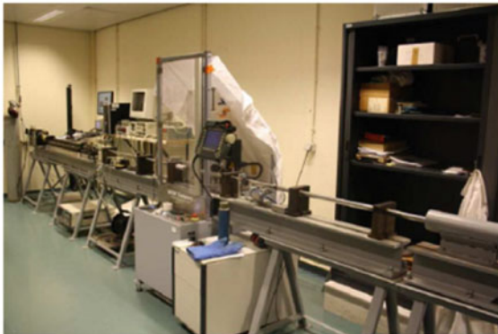
Fig. 1 The SHPB apparatus at the ballistic laboratory of the Royal Military Academy
