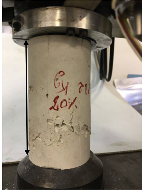
Fig. 4 GRC specimen after compressive test
