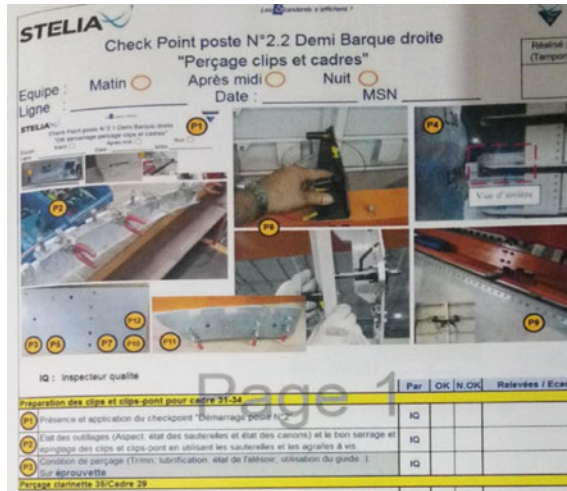
Fig. 7 Checkpoints extract of the assembly process of “right lower side of the fuselage”
