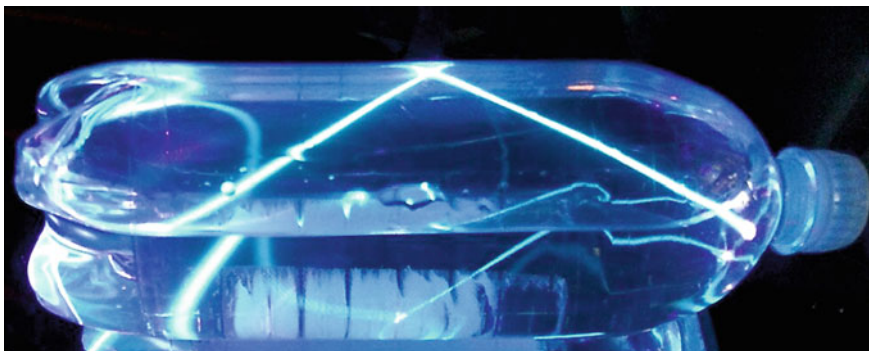
Fig. 7.9 Light from a blue-violet laser produces fluorescence as it passes through tonic water
