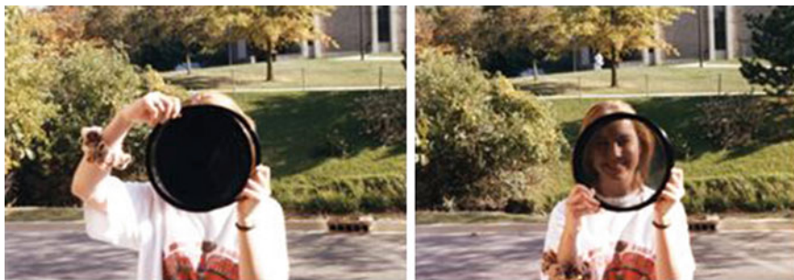
Fig. 6.3 Crossed and uncrossed Polaroid filters
