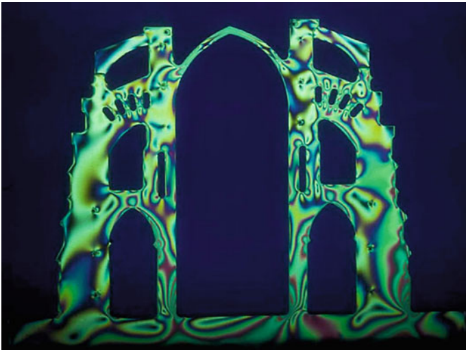
Fig. 6.12 Photoelastic model cross section of flying buttresses showing stress (Courtesy of Robert Mark)
