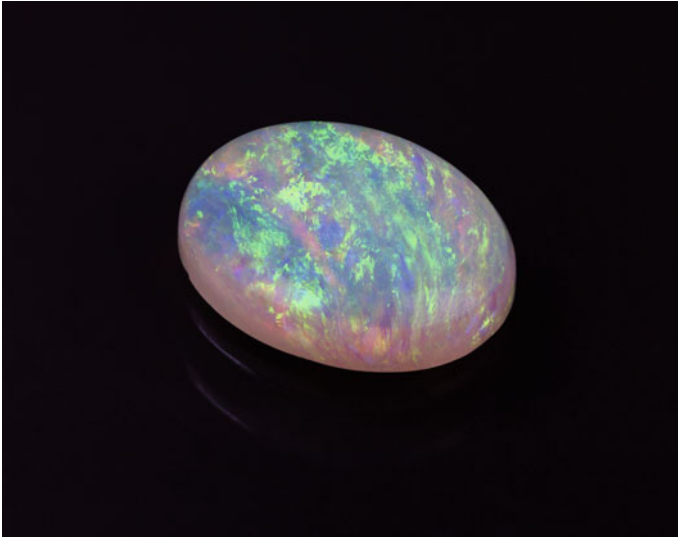
Fig. 5.26 An opal’s brilliance is due to light interacting with an ordered arrangement of silica spheres (TinaImages/Shutterstock.com)
