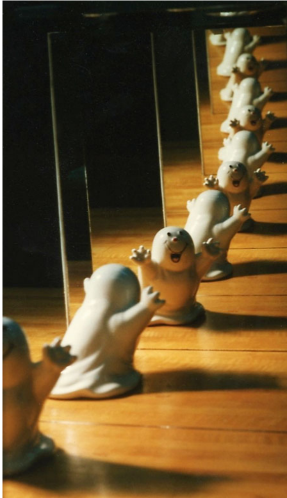
Fig. 3.28 Multiple images formed by two nearly parallel mirrors
