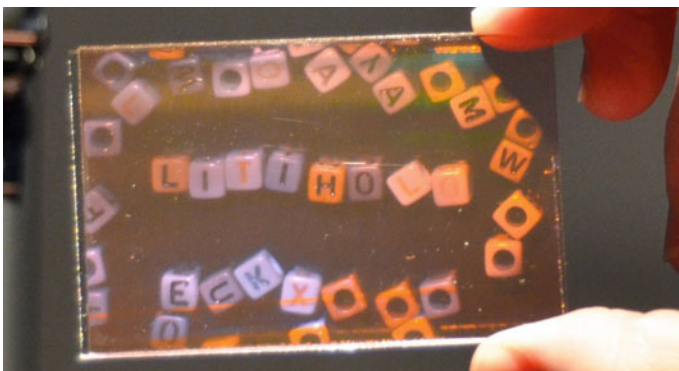
Fig. 11.12 A color hologram produced using red, green, and blue laser diodes and self-developing film (Courtesy of Litiholo)
