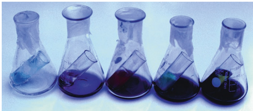
Fig. 7.12 Chromotropic acid spot test for formaldehyde in shampoos. Negative ( left ) and positive reactions (see explanations in text)
