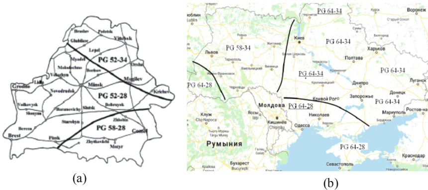
Fig. 1. Climatic zones according to Superpave method established for: (a) Republic of Belarus (b) Ukraine
