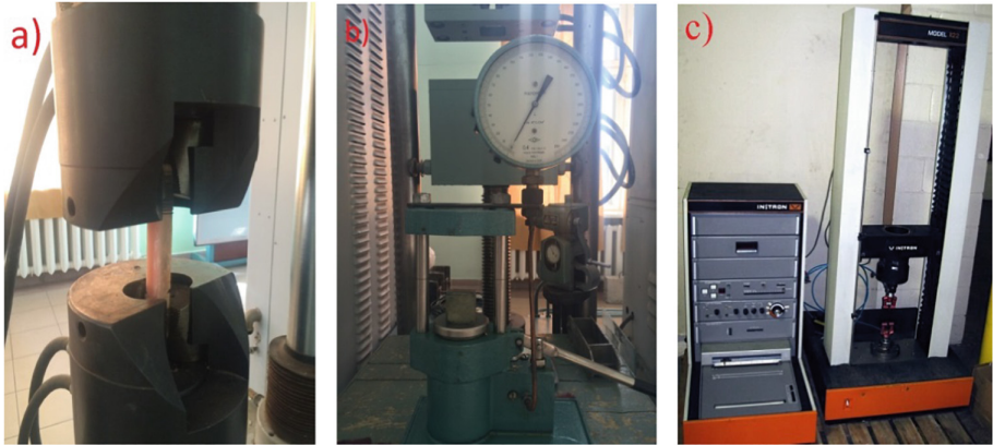
Fig. 1. Adhesive material block samples lab tests for constructing \sigma - \epsilon diagrams under the influence of tension (a), compression (b) and shear (c)
