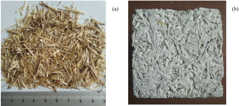
Fig. 1. Flax straw (a) and flax straw porous thermal insulation materials (b)
