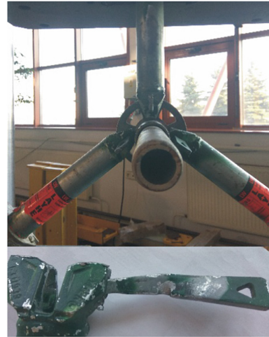
Fig. 8. Deformations of the whole joint and wedge.
