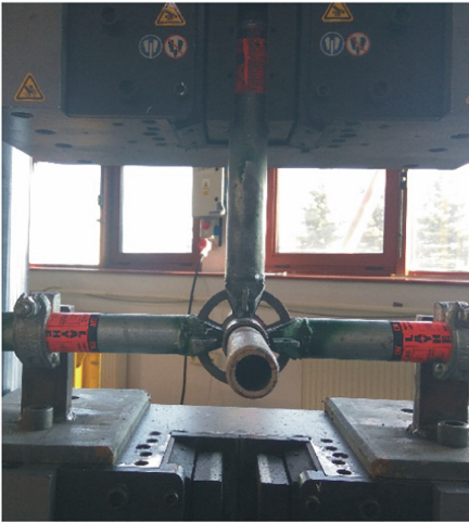
Fig. 7. Specimen on the test rig for bending of the joint in horizontal plane.
