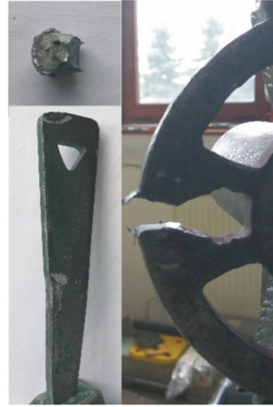
Fig. 2. Rosette sheared by the wedge.
