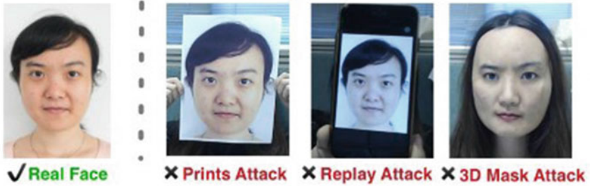
Fig. 1.9 Example of print, replay, and 3D mask attacks for face biometrics in mobile device [31]
