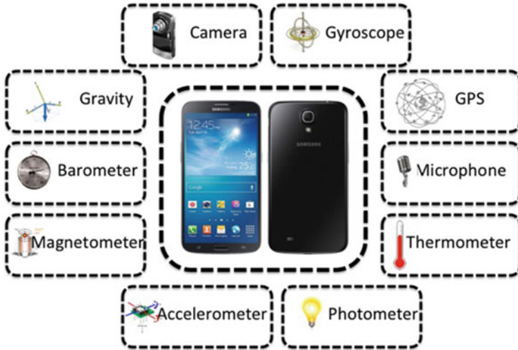
Fig. 12.2 Sensors and accessories available in a mobile device. Raw information collected by these sensors can be used to continuously authenticate a mobile device user
