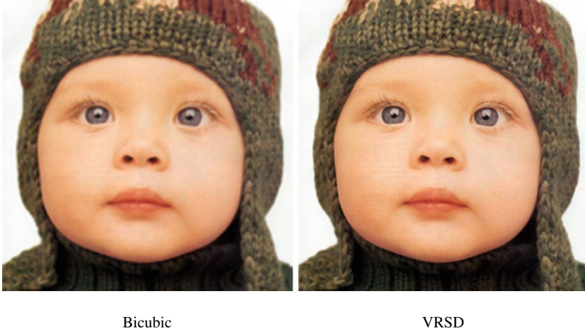
Fig. 5.2 Comparing the performance of a very deep CNN (VDSR) against bicubic interpolation
