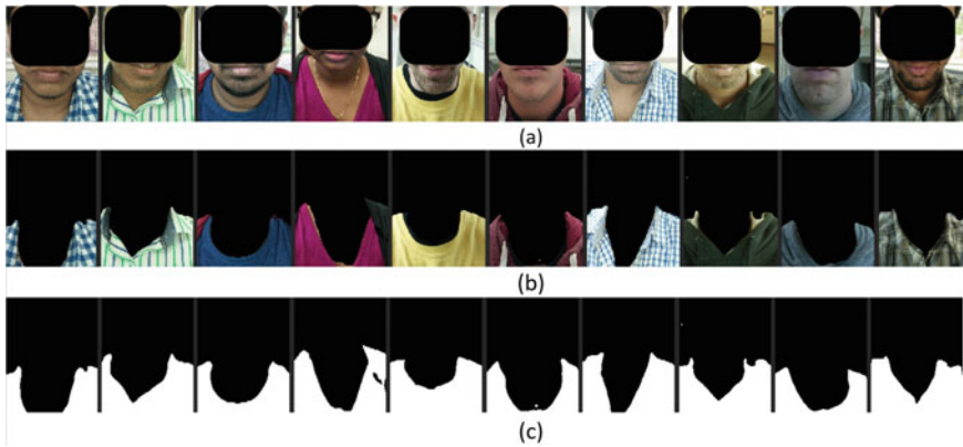
Fig. 13.5 Example of a original selfie images, b segmented clothes, c and the corresponding masks obtained by our U-Net model segmentation. The eye regions have been masked in order to preserve the privacy of the participants
