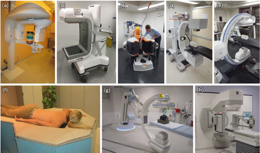
Fig. 2.2 Example CBCT systems. (a) CBCT for dental/ENT imaging (Carestream). (b) Mobile CBCT for image-guided ENT surgery. (Xoran; photo courtesy of Dr. R. Labadie, Vanderbilt University). (c) CBCT for imaging of musculoskeletal/orthopedic extremities (foot, ankle, knee, hand, wrist, or elbow; Carestream). (d) Prototype U-arm for CBCT of the head [32]. (e) Mobile C-arm
