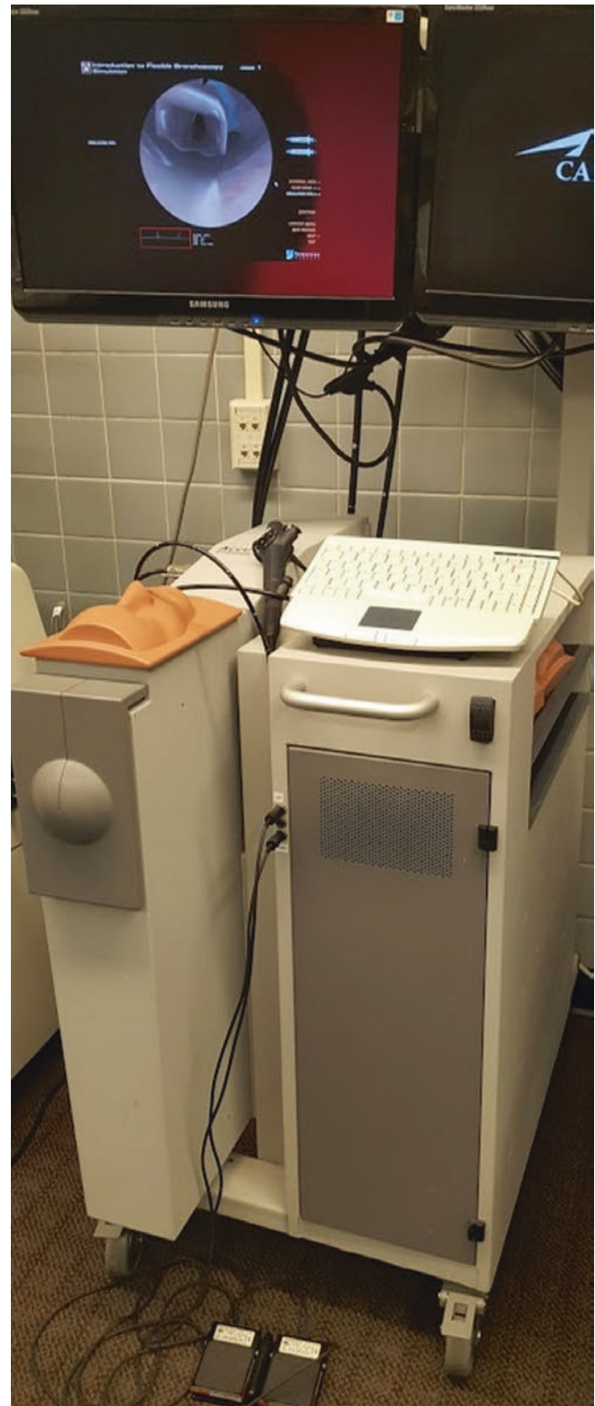
Fig. 17.5 A virtual reality bronchoscopy simulator (AccuTouch by Immersion Medical, Gaithersburg, Maryland) which consists of a flexible bronchoscope, a robotic interface with entry orifice, and a computer monitor with simulation software
