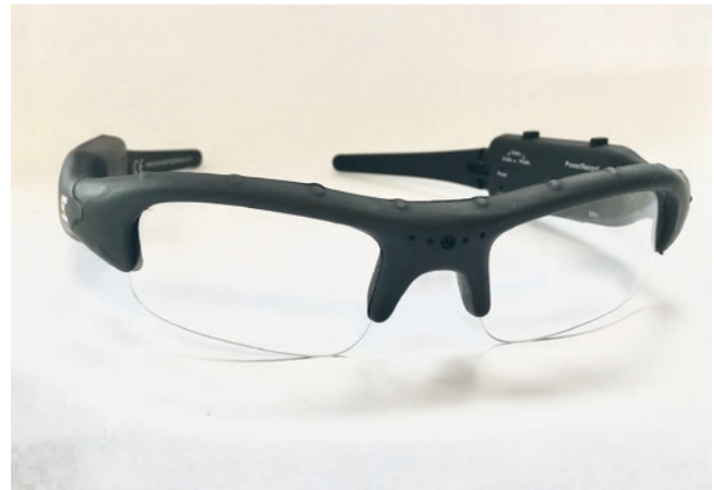
Fig. 12.1 Example of video glass to capture a research participants point of view (PoV) in an activity
