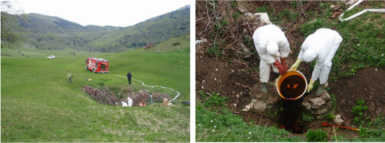
Fig. 7.2 Injection of uranine solution into the fissure at Malo Polje, 24 April 2014
