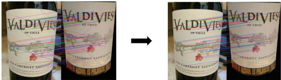
Fig. 4. The left and right subfigures illustrate the SIFT feature matching results without and with the RANSAC mechanism, respectively.
