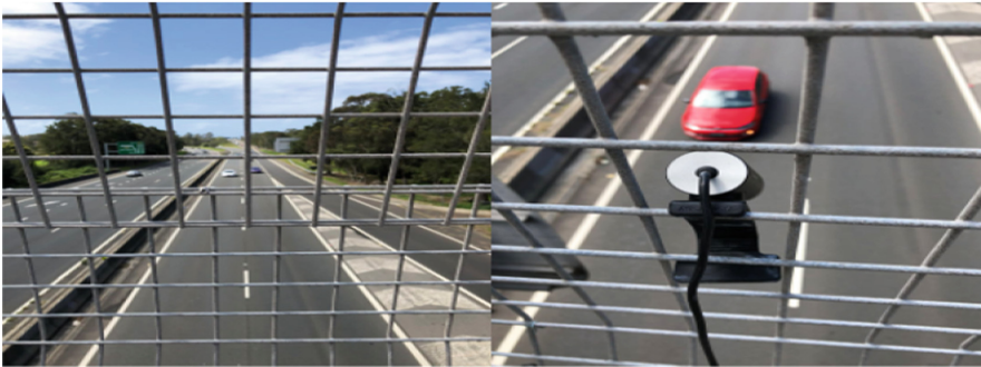
Fig. 5. Strategic placement of the camera above a highway. a. Urban stretch of road in Australia (left). b. Camera placement to avoid occlusion and count vehicles in real-time and estimate their speed (right).
