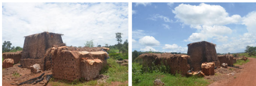
Fig. 3 Artisanal brick production from local laterite clay in the Mbarara region in Uganda
