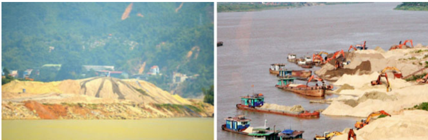
Fig. 1 Small scale industrial aggregates mining through river sand dredging in Vietnam; left: Son La river in Hoa Binh, right: Mekong delta
