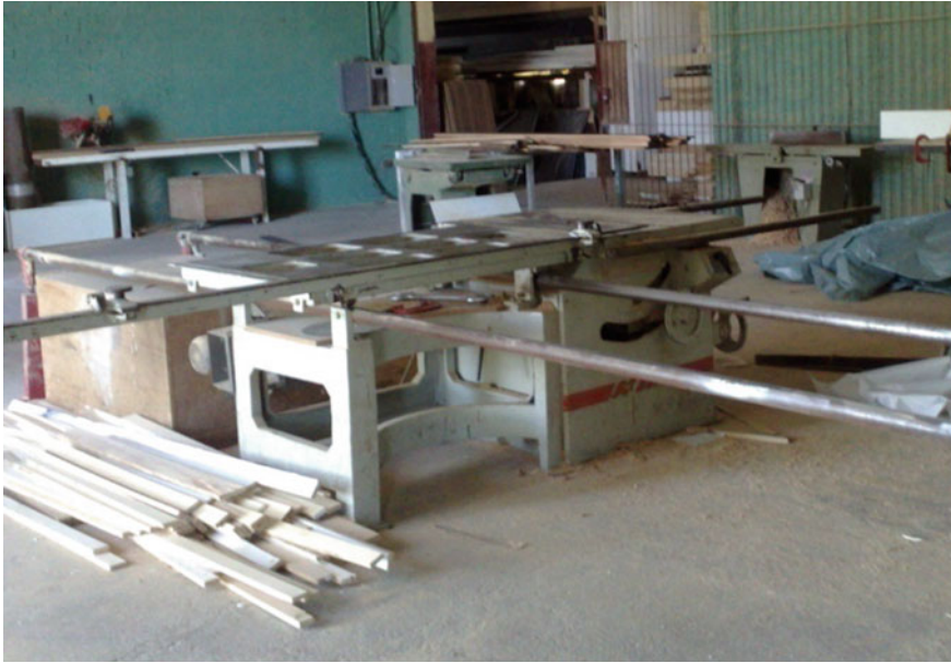
Fig. 2 Picture of the precision sliding table saw used in a joiner workstation
