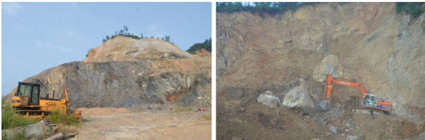
Fig. 2 Small scale industrial aggregates mining through hard rock and soil cover cutting in Hoa Binh province in Vietnam
