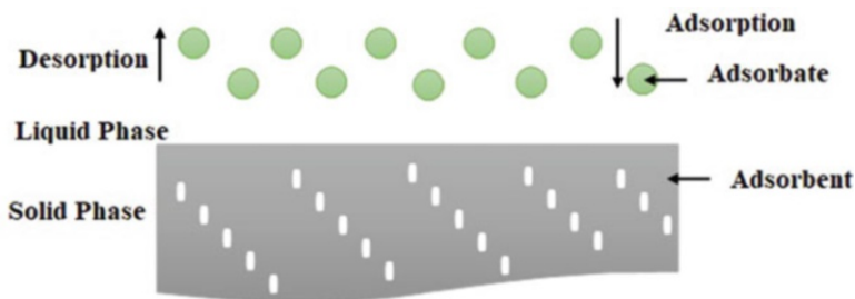
Fig. 1.1 Illustration of an adsorption terminology. Adsorption occurs when molecules in a liquid bind themselves to the surface of a solid substance. The adsorbate is accumulated on the adsorbent surface, and surface accumulation of adsorbate on an adsorbent is called adsorption
