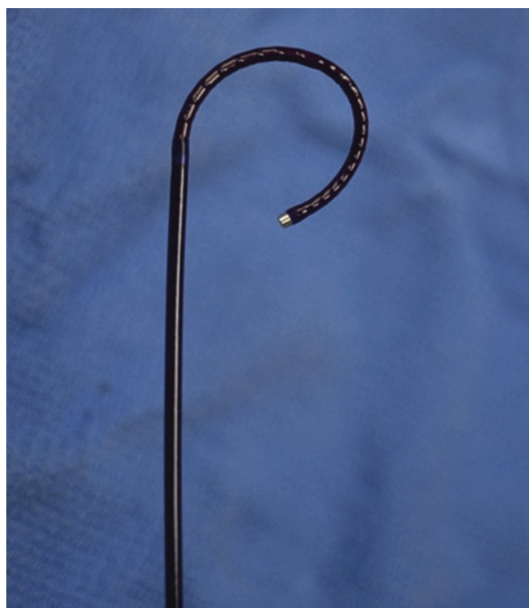
Fig. 1.4 The tip is deflected to approximately 220^\circ . This extent helps to correct for loss of deflection with an instrument in the channel
