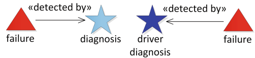
Fig. 6. Example of the SafeDeML::Diagnosis modeling with a system diagnosis (left) and a diagnosis perceived by the driver (right).
