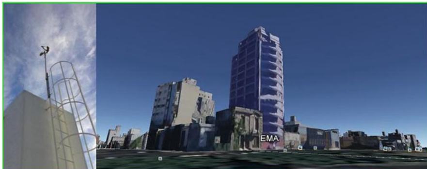
Fig. 12.12 (Left) Location of the anemometer on the water tank of the building; (right) the building and its surroundings where lower buildings can be seen
