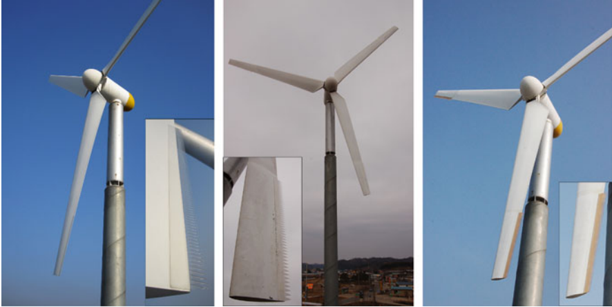
Fig. 14.7 Three different types of serration on blades [SNU]
