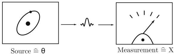
Fig. 18.1 Caricature of a quantum mechanical experiment. With every source of quantum systems, one associates a density matrix \theta . Observations systems are performed by measurement devices, which interact with incoming systems and produce real-valued outcomes. Each such devices is modelled mathematically by a Hermitian matrix X , referred to as an observable
