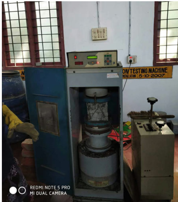
Fig. 1 Compressive strength test on fiber reinforced GPC
