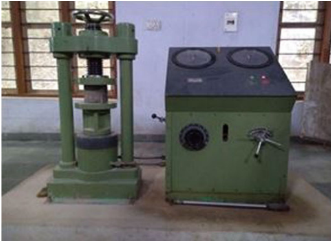
Fig. 5 Testing of mortar cube
