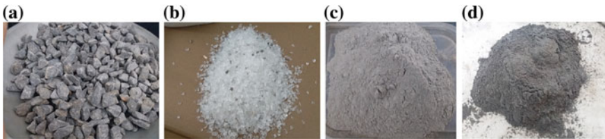
Fig. 2 Materials used a aggregate, b crushed glass, c fly ash, d rice husk ash
