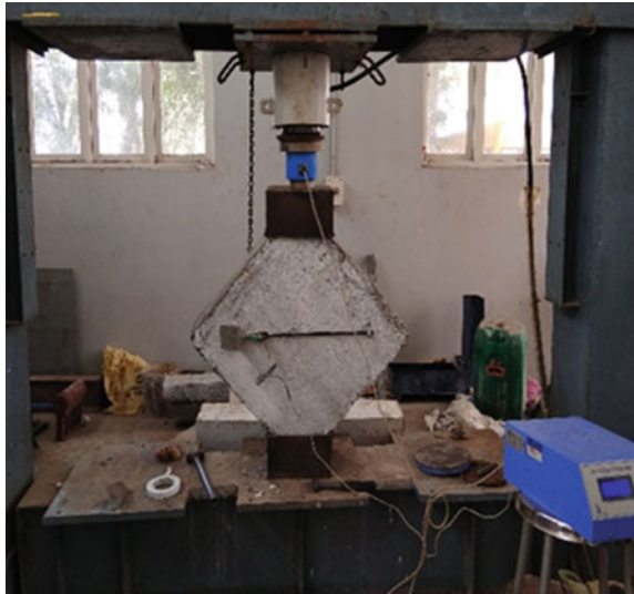
Fig. 6 Loading of concrete block panel
