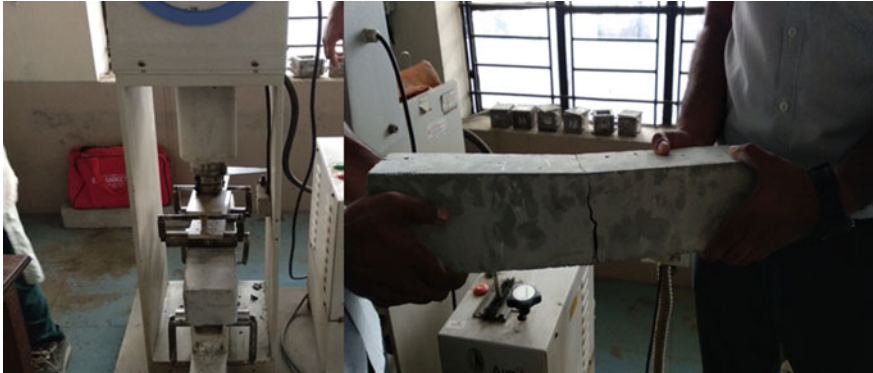
Fig. 5 Beam tested in flexural testing machine
