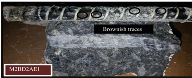
Fig. 6 Brown traces in BFRP embedded specimens
