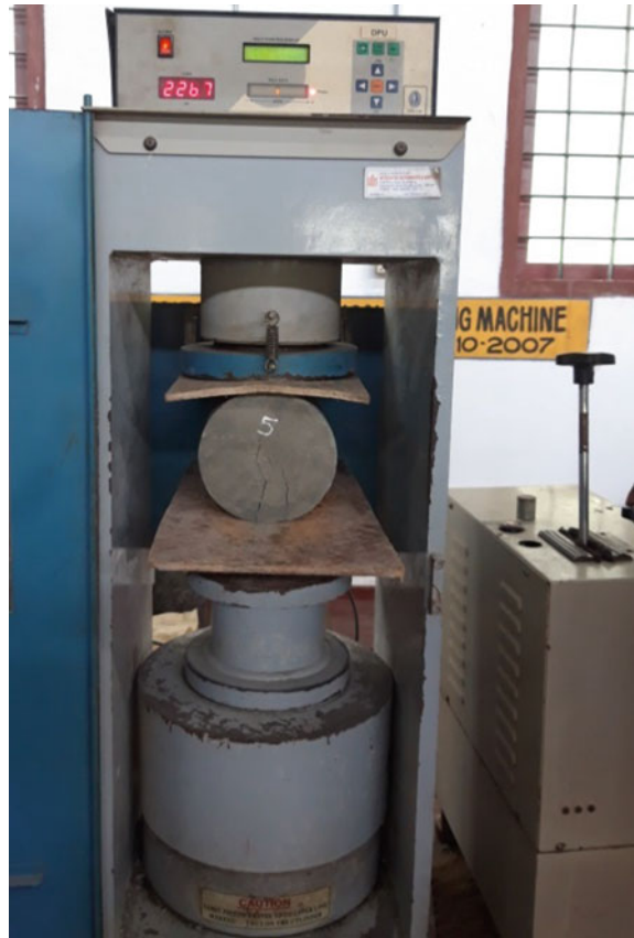
Fig. 3 Cylinder under split tensile test
