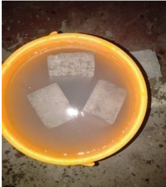
Fig. 9 Water absorption of bricks
