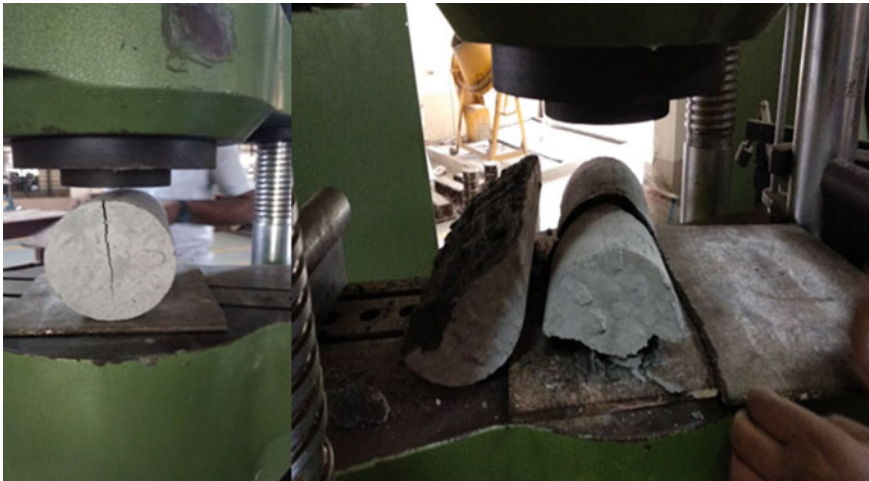
Fig. 3 Cylindrical specimens tested in UTM
