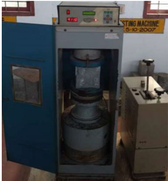
Fig. 2 Compressive strength test
