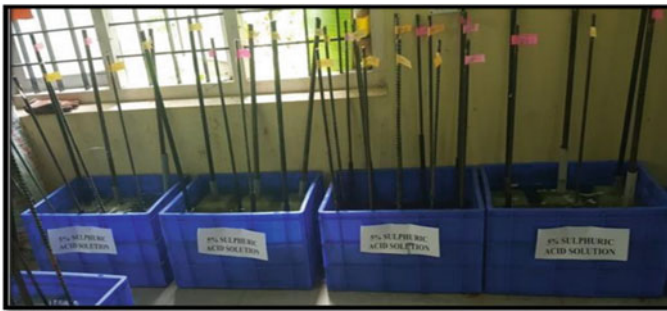
Fig. 4 Acid conditioning of specimens in crates
