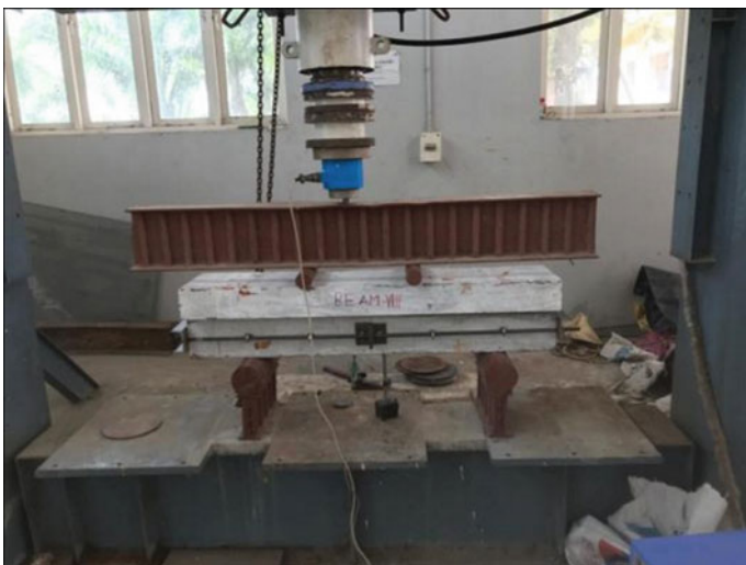
Fig. 2 Experimental setup of prestressed beams
