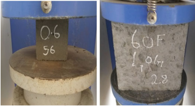
Fig. 1 Compression test setup of geopolymer concrete and mortar cubes
