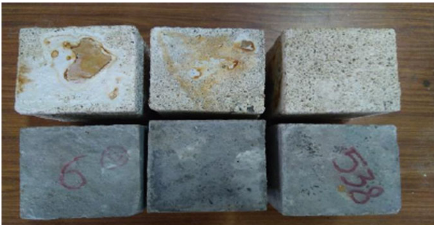
Fig. 9 Geopolymer concrete depicting lesser deterioration than conventional concrete
