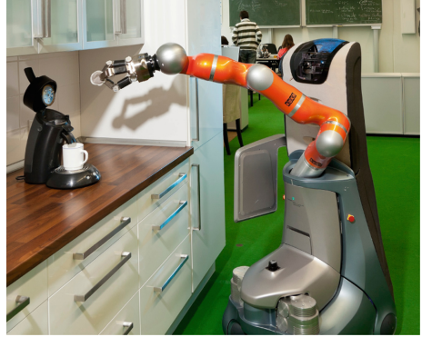
Fig. 1. The collaborative Care-O-bot 3 robot in a domestic environment.
