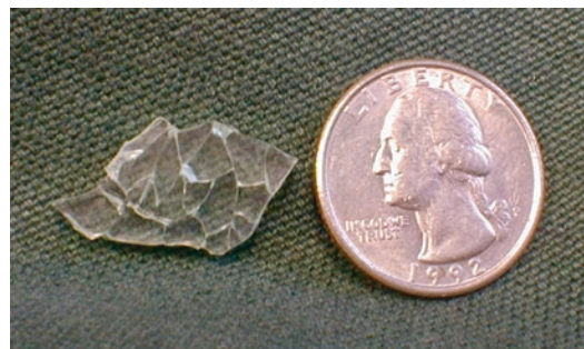
Fig. 44.5 Large shard of safety glass retrieved as an esophageal foreign body. The piece was too large to sheath inside the rigid esophagoscope to protect the esophageal mucosa. The special features of safety glass, however, helped to protect this infant. Safety glass fracture with mostly obtuse or square edges, decreasing the number of sharp knifelike edges that would have lacerated the esophagus. There was no injury to the esophagus upon retrieval of this foreign body
