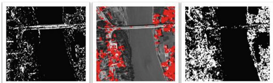
Fig. 2. (Left to Right) Applied Harris on a gray image, R1 (Edges but not corner) and Applied Peaks
