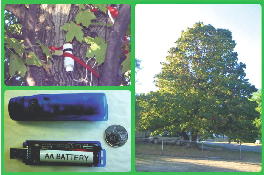
Fig. 6.6 Accelerometer and waterproof enclosure installed on sugar maple tree (top left), X-16C accelerometer with U.S. quarter shown for scale (bottom left), and full-sized maple tree employed in these experiments (right). The TDR probe is adjacent to the accelerometer and above it approximately 0.35 m, although not pictured
